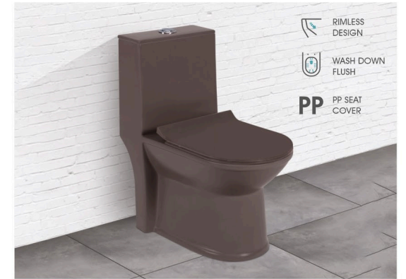
LEXUS-S/P-CHOCO (Matt) L 690 W 375 H 750 S Trap - 225mm(9") | P Trap - 175mm
